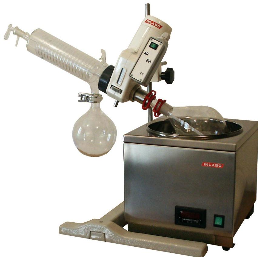
**Rotary Evaporator EVI 67/1 with WATER BATH EVI 91**
